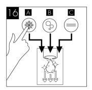
When the external cleaning (minimum 5 minutes) is completed, flush the machine using the chilled button with clean water until the dispense water runs clear. Repeat briefly with the ambient and sparkling buttons if present.
