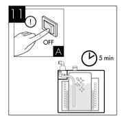
Leave the solution inside machine for sanitisation to take effect (minimum 5 minutes) while thoroughly cleaning the dispenser externally. (All maintenance operations must be carried out with the dispenser switched off.)
