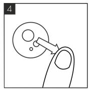
Ensure to release the Sparkling water button and take care to avoid releasing excess amounts of CO2 gas as this may damage the tank.
