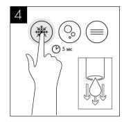
Briefly press chilled dispense button to release internal water pressure from the machine.
