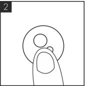
Press and hold the Sparkling water dispense button until all the water is expelled and only CO2 gas is being released.
