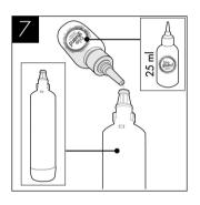
Add 25 ml of Bioguard Internal Sanitising Solution to a clean and empty service filter cartridge.
