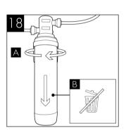
Remove the service filter. Retain service filter for reuse.
