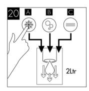
Pre-flush the new filter to waste using the chilled button until the water appears clear and is free of air. Flush through a small amount of water to check all functions.
