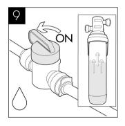
Turn on incoming water, allow the service filter cartridge to fill
